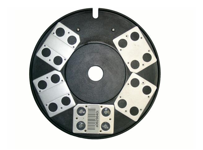
When **TLD chips** and/or. **TLD- sticks** are calibrated, you take the plate with the blind holes arranged at the edge (combi disc), into which the elements are to be put down.
