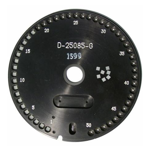
Then the thrust subject is put to be pulled out up to the notice and the appropriate plate is put on the thorn. It is to be noted that the follower pin of the equipmentfirm mother board sits in the groove of the plate. Otherwise the plate is to be turned so for a long time, until the pin engages.
