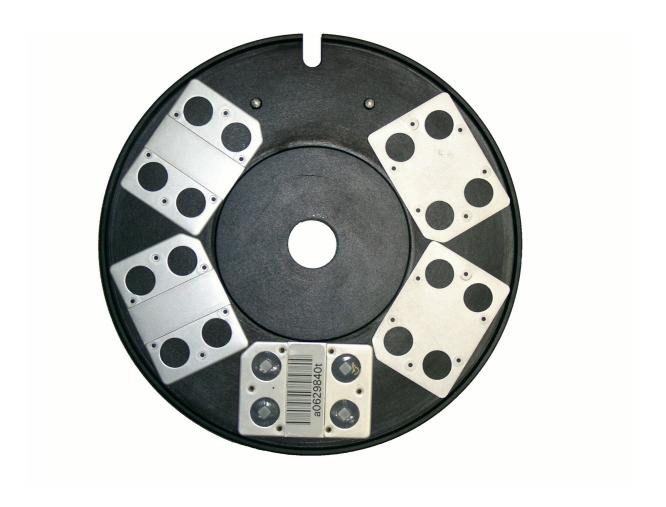
When **TLD chips** and/or. **TLD- sticks** are calibrated, you take the plate with the blind holes arranged at the edge (combi disc), into which the elements are to be put down.
