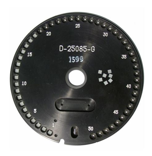
Then the thrust subject is put to be pulled out up to the notice and the appropriate plate is put on the thorn. It is to be noted that the follower pin of the equipmentfirm mother board sits in the groove of the plate. Otherwise the plate is to be turned so for a long time, until the pin engages.
